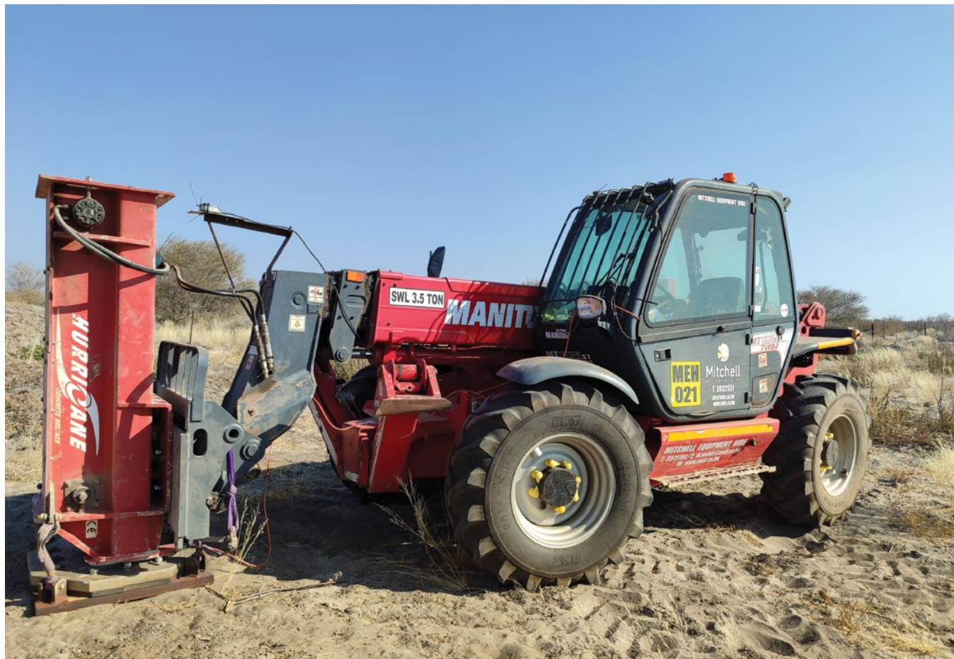
Figure 2: Weight drop for active seismics at KITW
