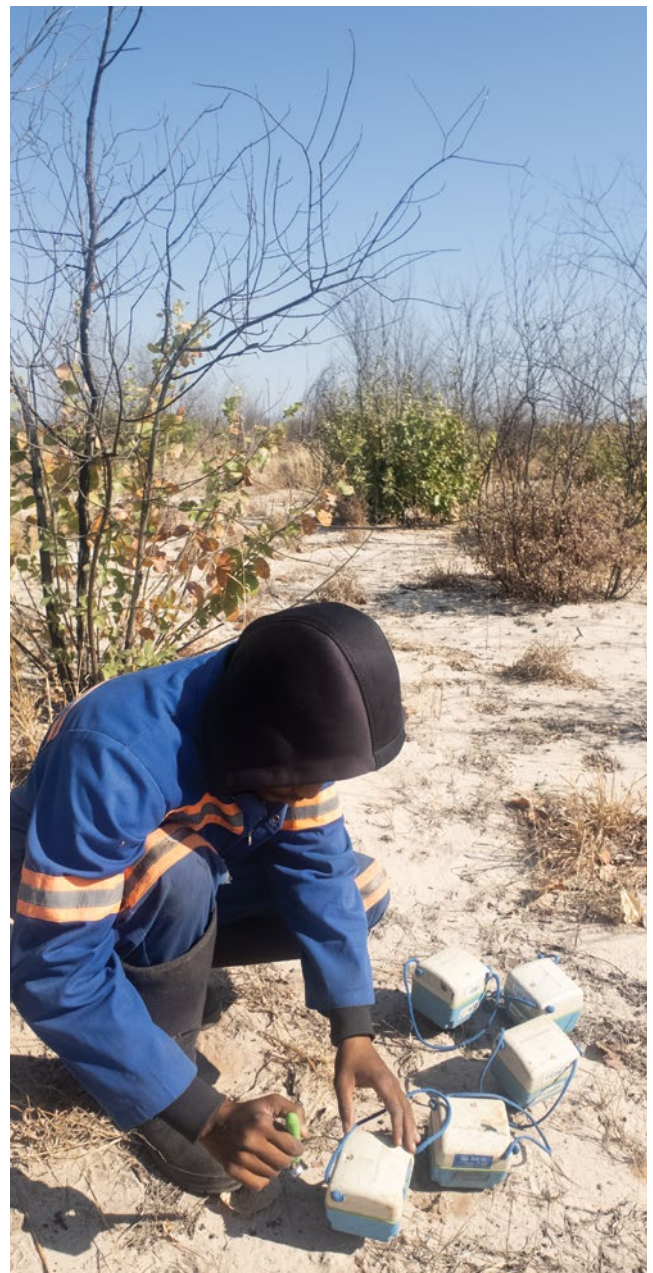
Figure 1: Passive seismic node deployment at KITW
