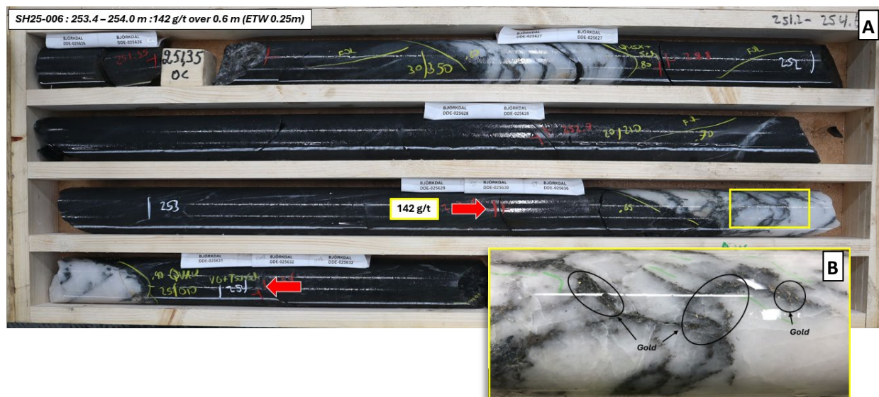
Figure 4. Drill core photos from SH25-006 showing an intercept grading 142 g/t gold over 0.60 m (ETW 0.25 m) (A) and a close-up of mineralised quartz vein (B).
