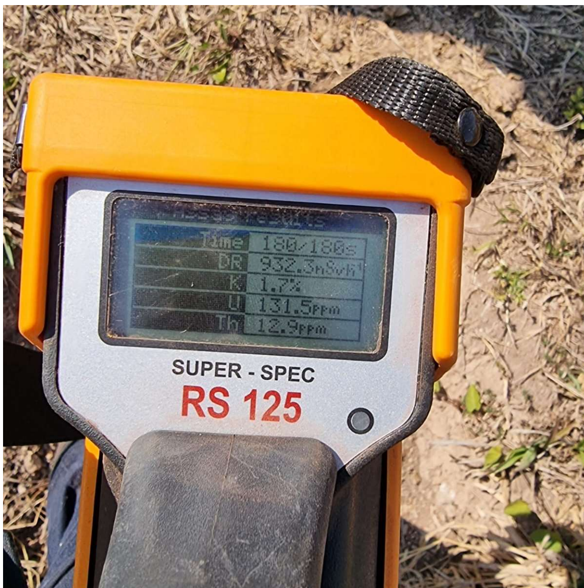
Figure 3. Spectral Scintillometer reading from Prospect 1 (NE corner of Figure 2) showing individual readings for Uranium, Thorium and Potassium using the “assay” function of the device. NB. Surface soil sample, not outcrop.
