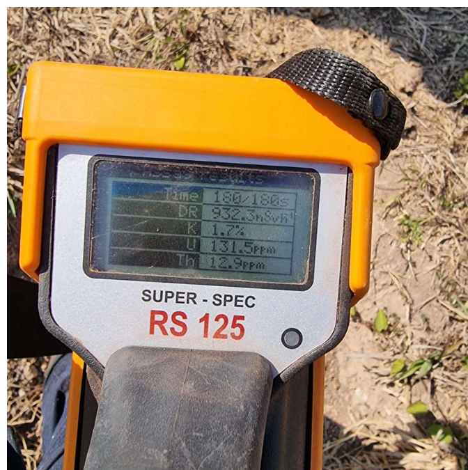
Figure 7: Spectral Scintillometer reading from Prospect 1 (NE corner of Figure 2) showing individual readings for Uranium, Thorium and Potassium using the "assay" function of the device. NB. Surface soil sample, not outcrop
