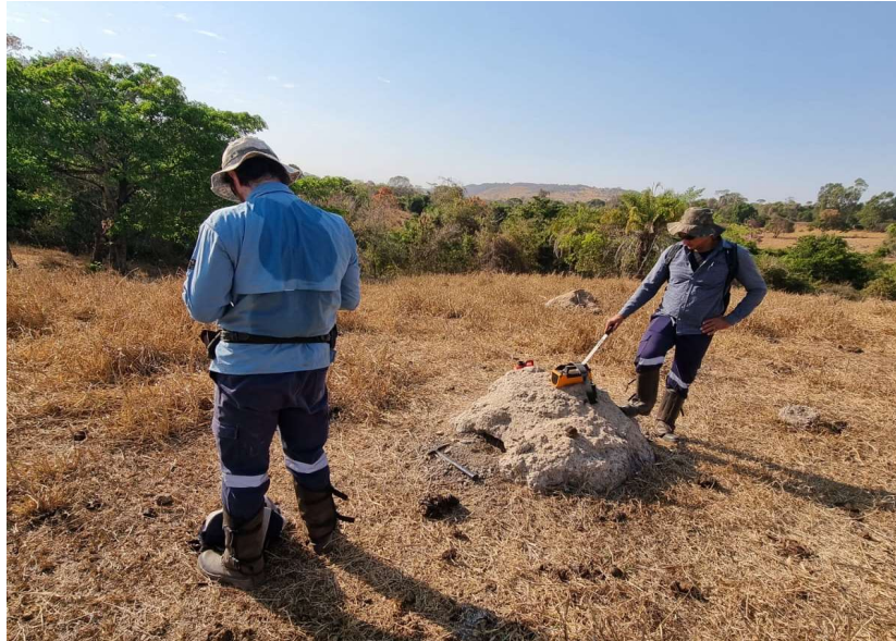
Figure 6: OAR field team on site at Amorinópolis mapping and using the RS-125 Spectral Scintillometer to gather and assess the radioactive readings of the outcropping sandstone units
