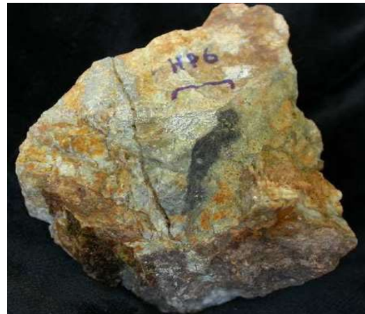
Sample AG(1)* 4 (Petrographic sample HP6), 17.9ppm Gold (Au) and 6.2ppm Silver (Ag), not assayed for Antimony. Breccia-vein material of quartz-arsenopyrite (scoroditised)-pyrite-very minor chalcopyrites); Sample: 20cm block broken off large embedded boulder, possibly outcrop, (from EL5339 now EL9293) (cm scale bar drawn on specimen). Sample collected by M. Leu around coordinate 3000N 7393.5E based on Amoco's grid. Results reported in ALS Certificate of Analyses ST37207 – 2003.
