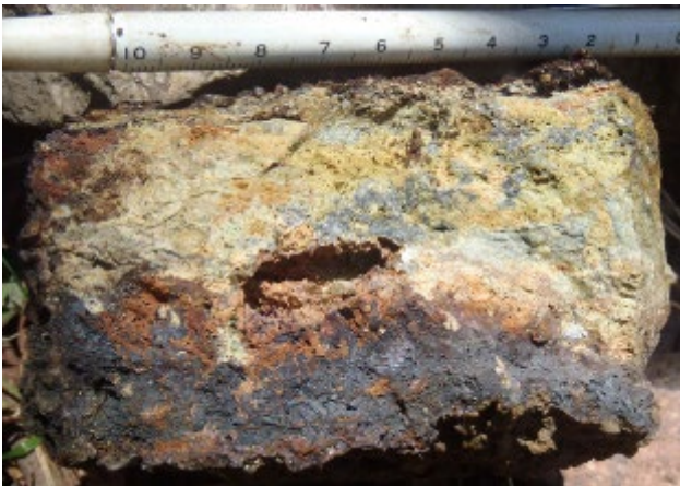
Sample S671* 5 , 12.9ppm Gold (Au), 0.53% Antimony (Sb) and 18.5ppm Silver (Ag). Vein composed of brecciated quartz-arsenopyrite (scorodite)-quartz-brecciated metasediments (protolith siltstone); Sample: float, (from EL5339 now EL9293) (Ruler: cm). Sample collected by M. Leu around coordinate 3000N 7700-7600E based on Amoco's grid. Results reported in Certificate of Analyses BR12233601 – finalised 25 10 2012.
