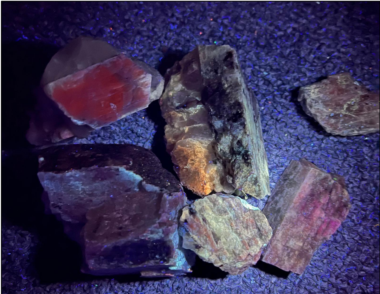
Figure 2 – Field samples from the Tango Lithium Project (Island Showing) being checked under fluorescent light 1
