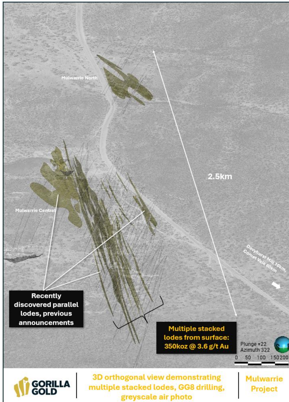
Figure 3. Oblique 3D view of Mulwarrie, demonstrating the scale of the system with multiple lodes from surface over a zone ~200m wide by greater than 2km long.
