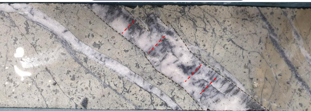
Quartz-carbonate-stibnite extension veins in altered dyke
