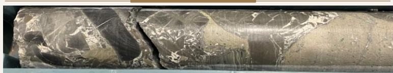
SDDSC079, 548 m; Complex dyke-sediment interaction, with dyke fragments (beige), altered and unaltered sediment fragments, with partial quartz vein matrix.
