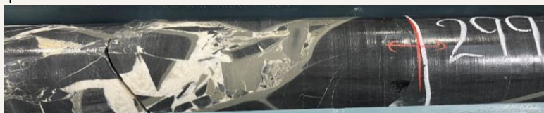
SDDSC106, 299.8 m; quartz-vein matrixed dyke breccia, with angular sediment and altered sediment fragments with quartz vein-breccia matrix
