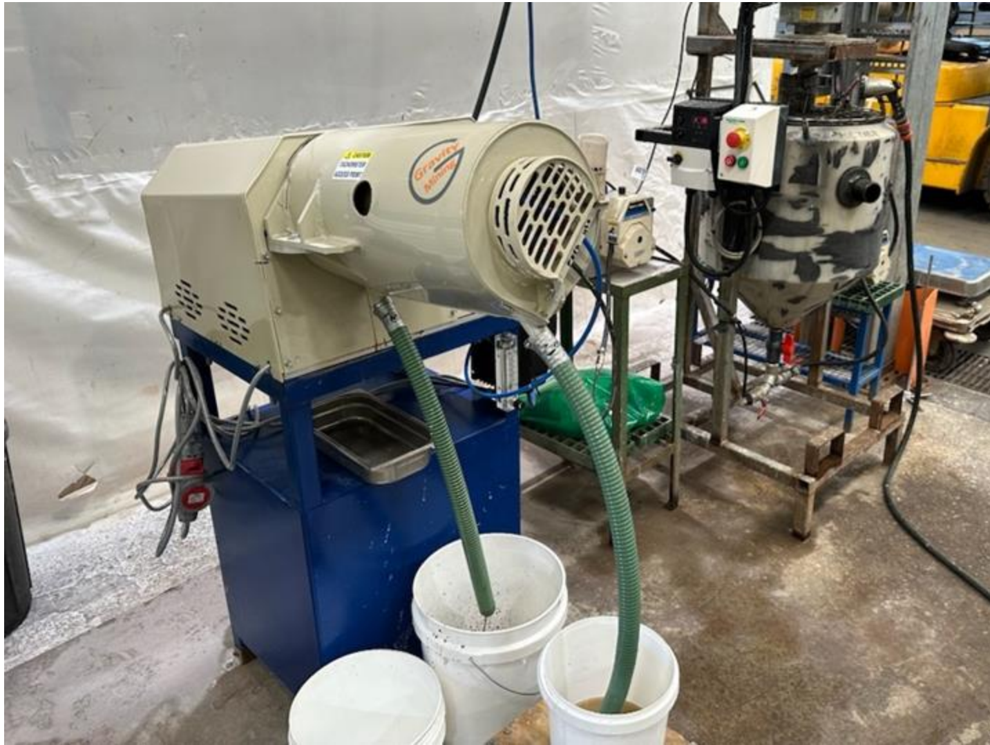
Laboratory-scale, multi-gravity separator (MGS) testing with Sandy Mitchell HMC
