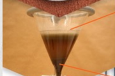
Photo 5. Laboratory HM separation via a heavy liquid
