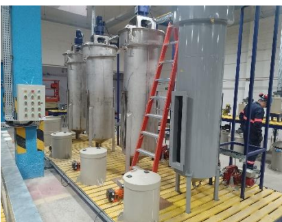
Figure 3: Counter Current Decantation (CCD) circuit
