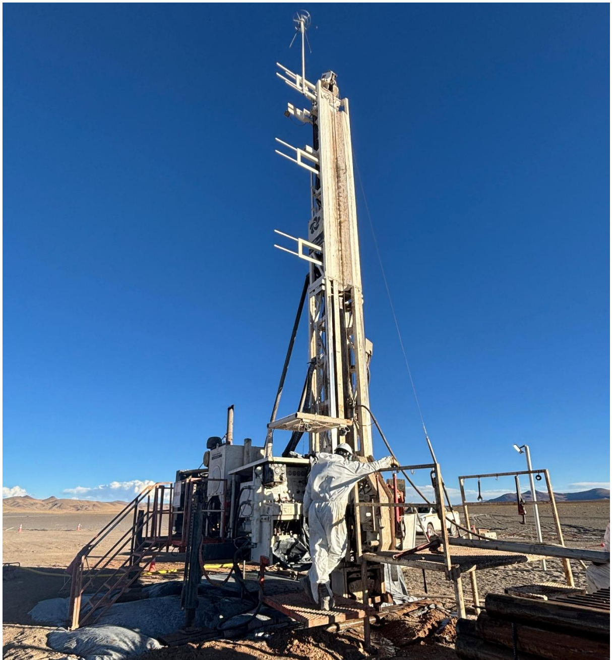
Figure 1. Boart Longyear Core Drill LF-140 rig at JAM 25-05 drilling first 30m for steel casing.
