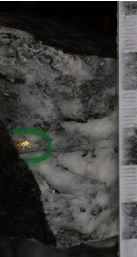
NSD057 – 108.2-109m includes multiple instances of visible gold (VG) in quartz veining. This is not typical for Stawell – and the geology, mineralisation and structure have strong similarities to the historic Mariners mines that boasted an historic production grade of ~30 g/t Au (see p. 11 for details on Mariners).
