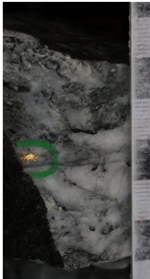
NSD057 – 108.2-109m includes multiple instances of visible gold (VG) in quartz veining. This is not typical for Stawell – and the geology, mineralisation and structure have strong similarities to the historic Mariners mines that boasted an historic production grade of ~30 g/t Au (see p. 11 for details on Mariners).
