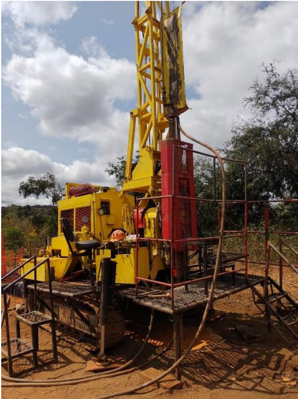
Figure 5: Diamond drill rig in operation at Caladão Project Phase 1 drill program
