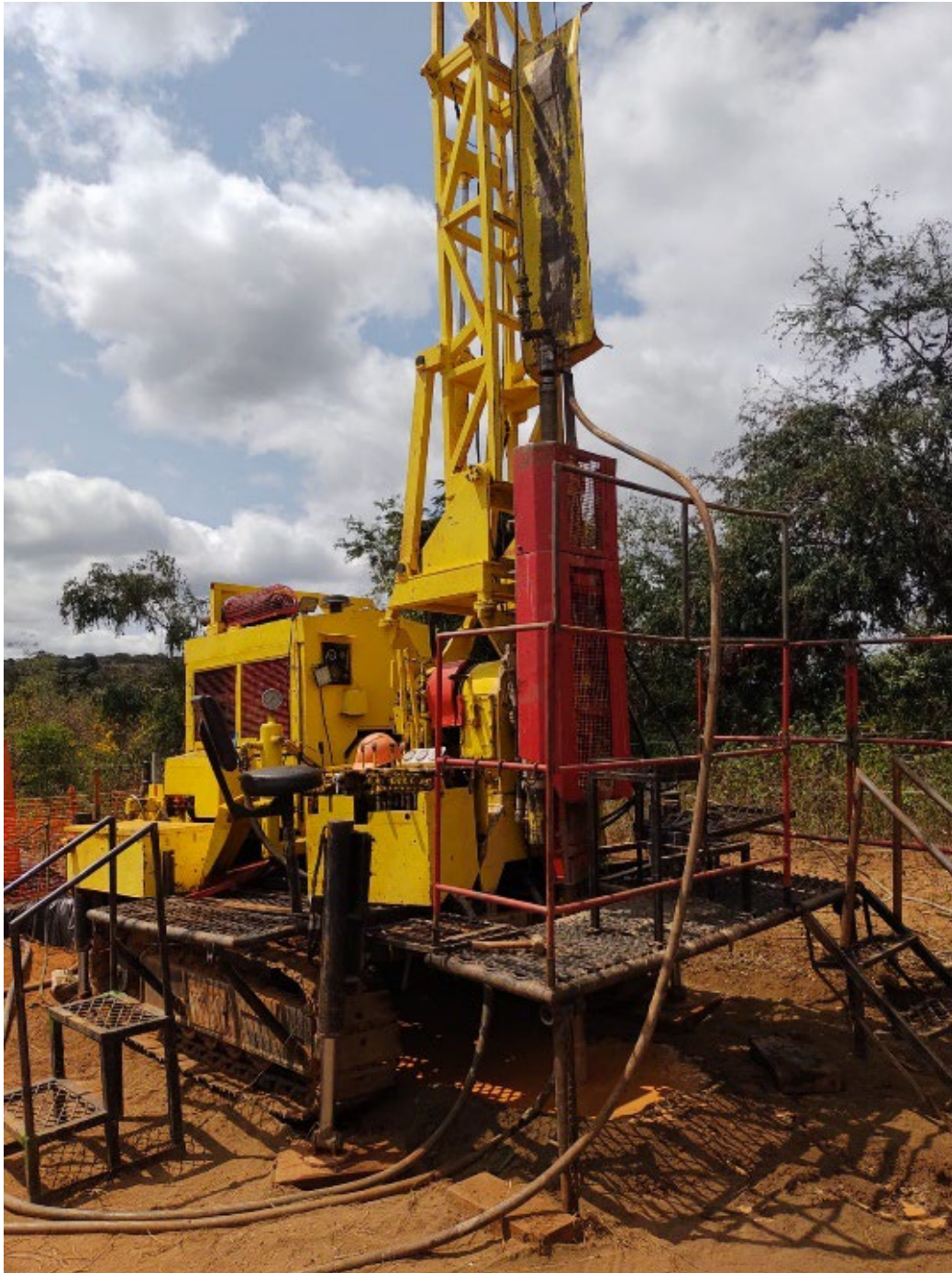
Figure 3: Diamond drill rig in operation at Caladão Project Phase 1 drill program
