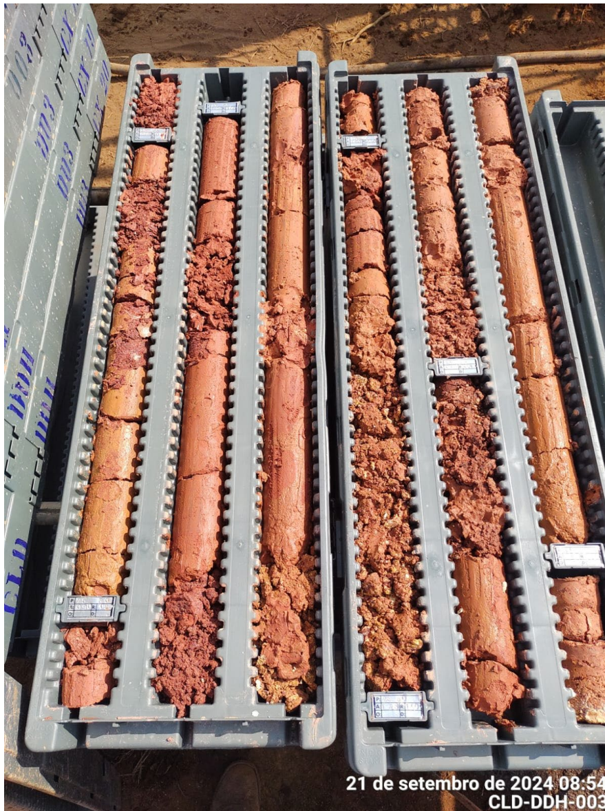
Figure 4: Caladão Project diamond drill core tray (CLD-DDH-003 ) showing thick kaolinite-rich weathering profile.
