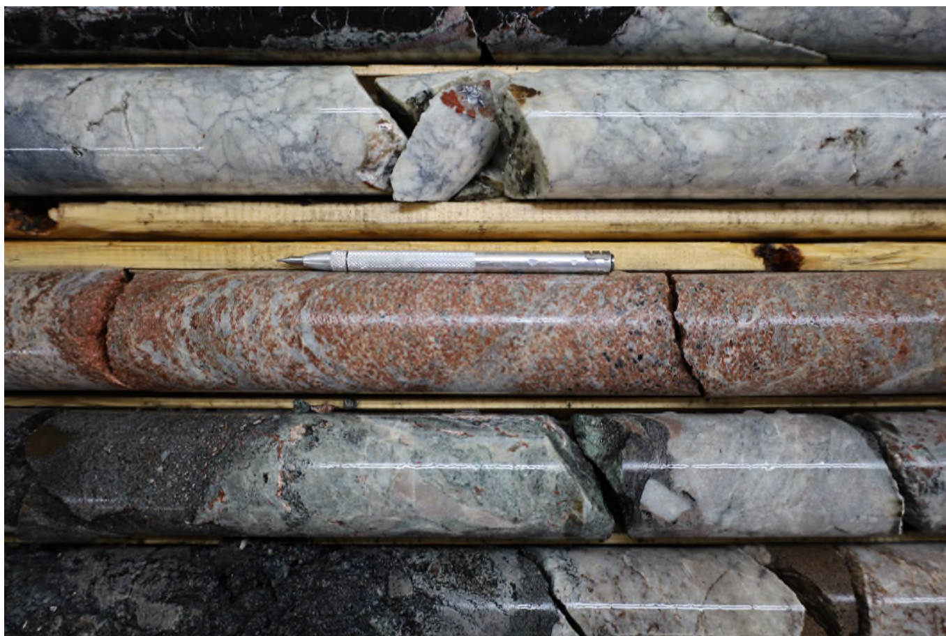
Figure 4: Diamond drill core (NQ, approximately 4.8 cm diameter) containing strong REE mineralisation (red coloured disseminations to semi-massive) within ferrocarbonatite/calciocarbonatite host rock. Hole POM-23-03, 173m downhole depth.
