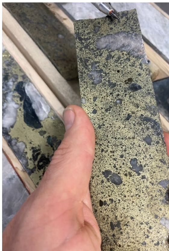
Figure 2: High grade drill core from CB-24-100 intersecting 7.3m @ 4.2% Cu, 0.3g/t Au & 16.6g/t Ag at Corner Bay. Image showing core between 321.9m and 322.6m.
