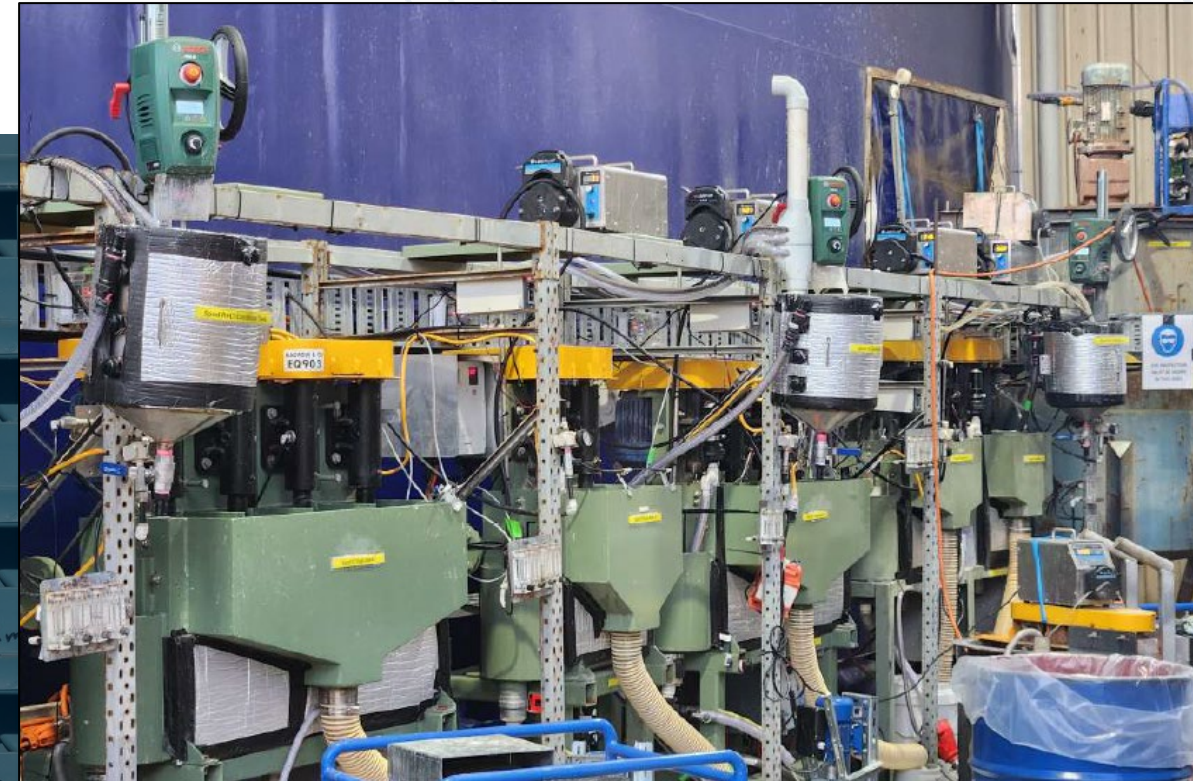
Pilot plant spodumene flotation circuit during operation
