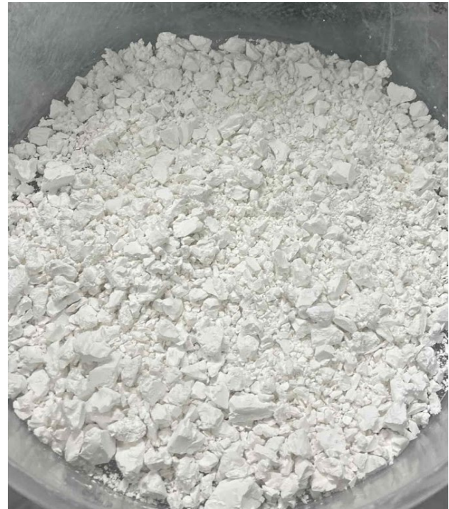
Figure 3: Hydrated niobium oxide precipitate (before calcination)
