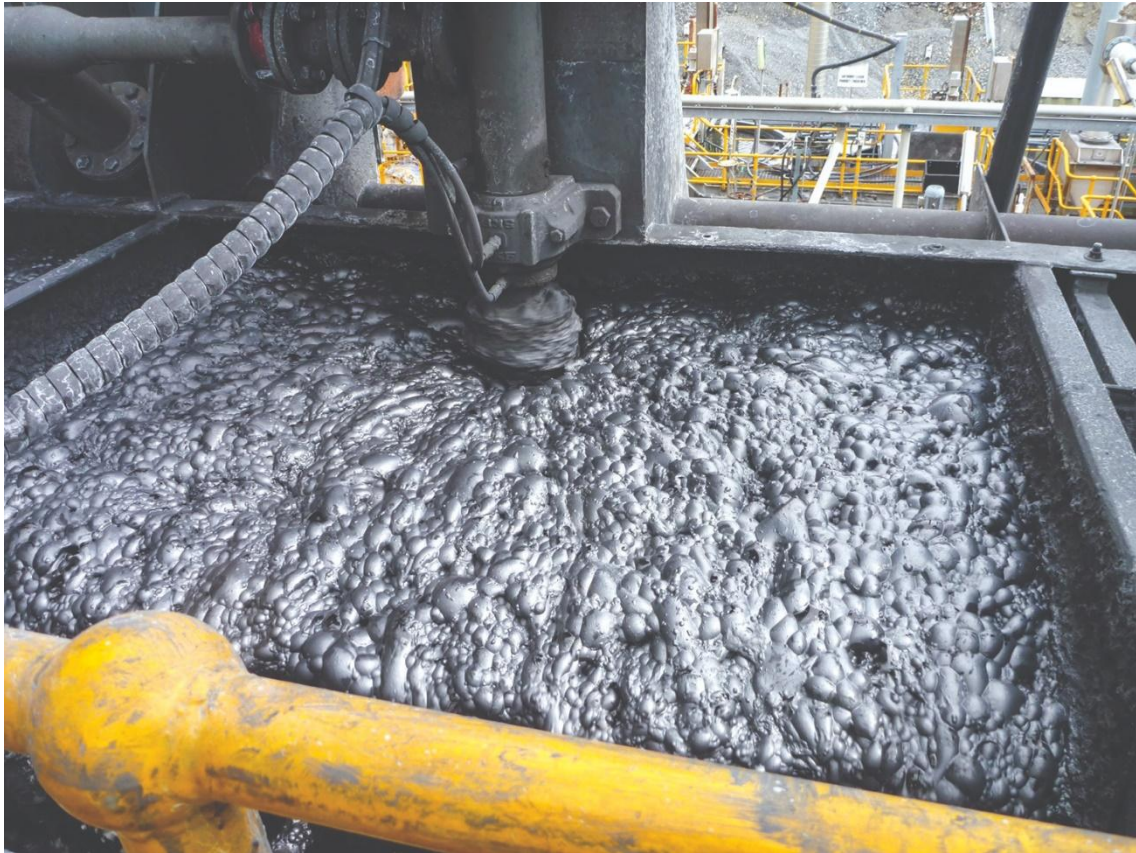
Figure 1: Mineral Hill flotation processing.
