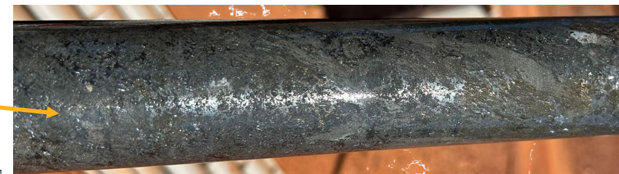
Core from drillhole EHDD25001 (~240m depth) showing semi-massive sulphide mineralisation (pyrite-pyrrhotite-boulangerite ( Pb_5Sb_4S_{11} ))
