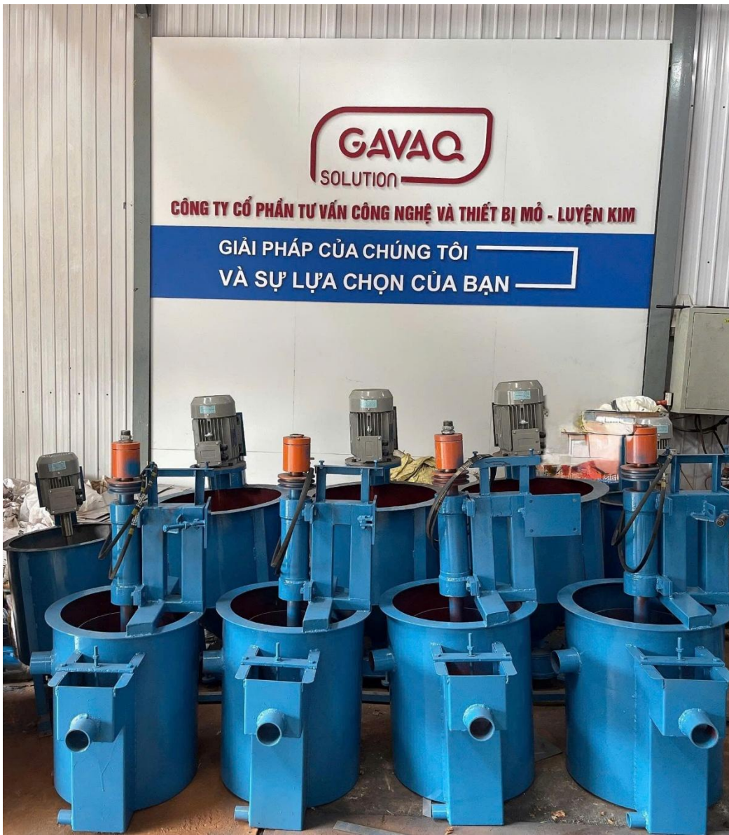
Image 3 – Pilot Plant equipment arriving (Flotation Cells)
