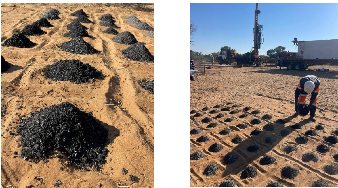
Figure 3 - Serowe-3.4A Drilling Operations and Rock Chip Sampling (Source: Botala)
