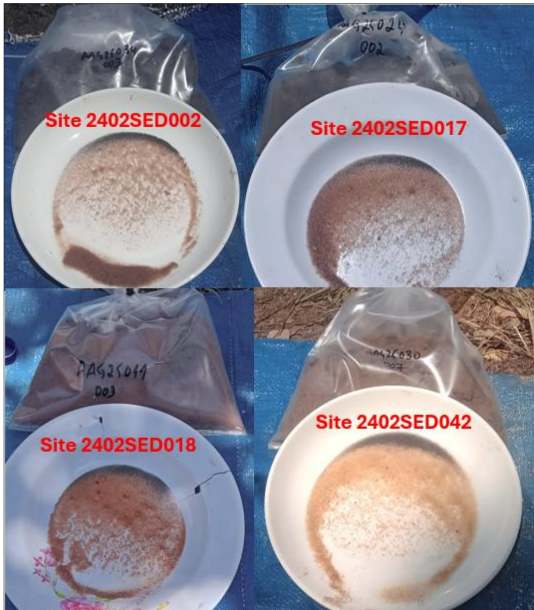
Figure 1: Panned Heavy Mineral Concentrate (HMC) samples from drill samples within each of the four (4) drilled areas within Adriano (11002L).
