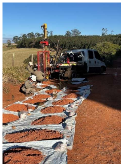
Figure 1: Images illustrating the hydraulic auger drilling process, the systematic collection and arrangement of soil samples for detailed field description.
