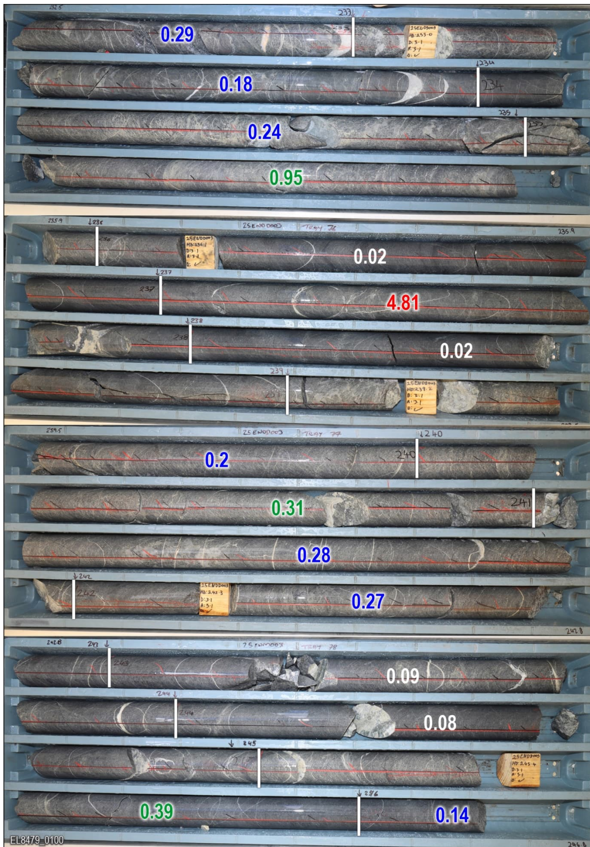
Photo 2. Core tray photos of 25ENDD003 interval 44m @ 1.77g/t Au from 235m incl. 9.7m @ 3.57g/t Au from 252.3m. Distinctive paler coloured zones (silica-sericite altered) typically host better grades (although not exclusively) and are interpreted to have overprinted the darker coloured zones (propylitic/chlorite altered). The numbers superimposed on the core are the reported gold assay grades over each respective sample interval.
