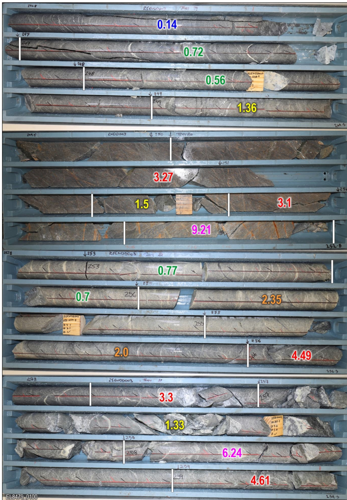
Photo 2 (continued from previous page). Core tray photos of 25ENDD003 interval 44m @ 1.77g/t Au from 235m incl. 9.7m @ 3.57g/t Au from 252.3m. Distinctive paler coloured zones (silica-sericite altered) typically host better grades (although not exclusively) and are interpreted to have overprinted the darker coloured zones (propylitic/chlorite altered). The numbers superimposed on the core are the reported gold assay grades over each respective sample interval.
