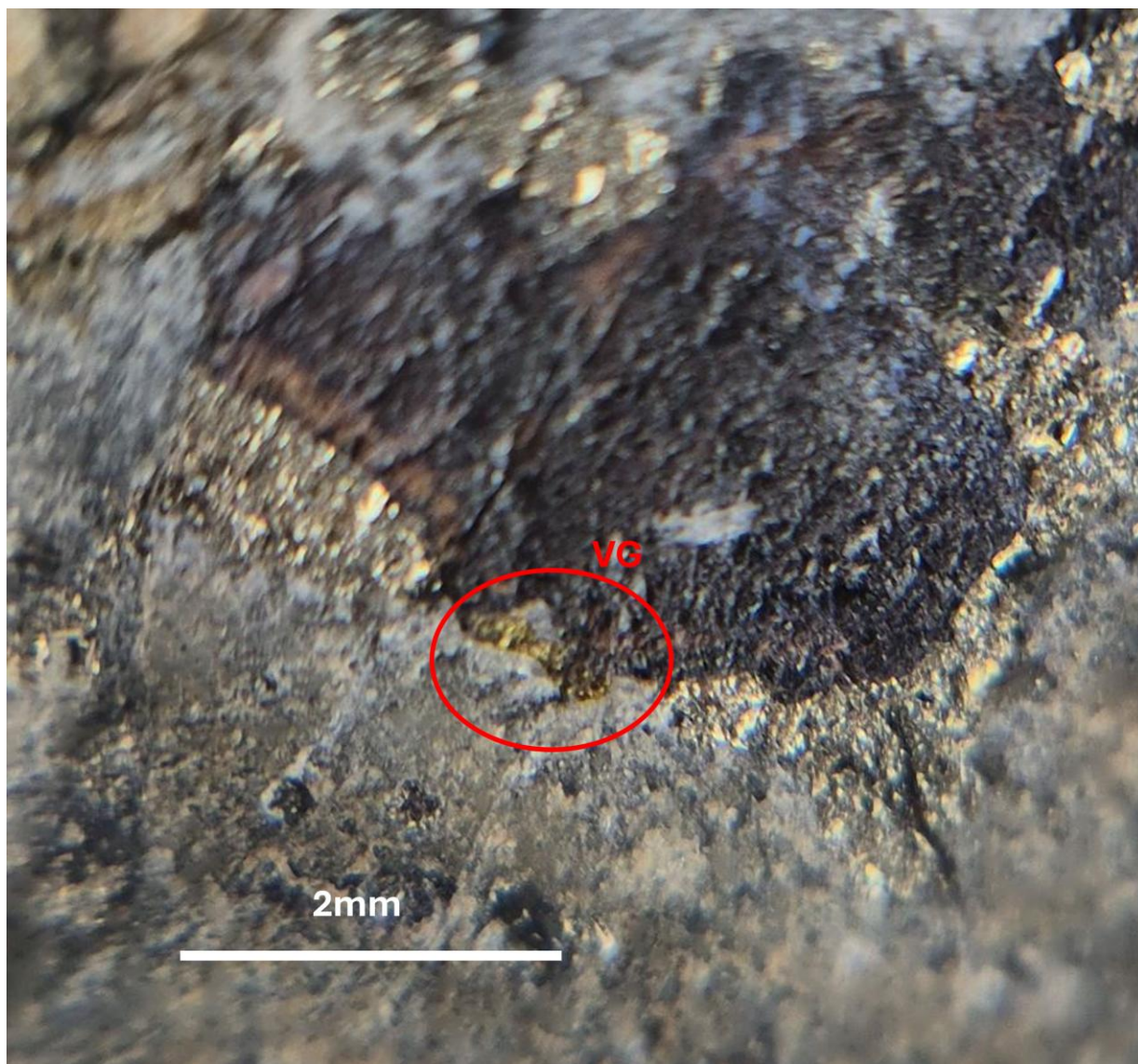
Figure 1: Photograph through magnifying camera lens showing visible gold (vg) on the edge of a sphalerite clast observed in ZRMDD066 within interval of 0.5m @ 19.8g/t Au from 394.90m in granitoid.
