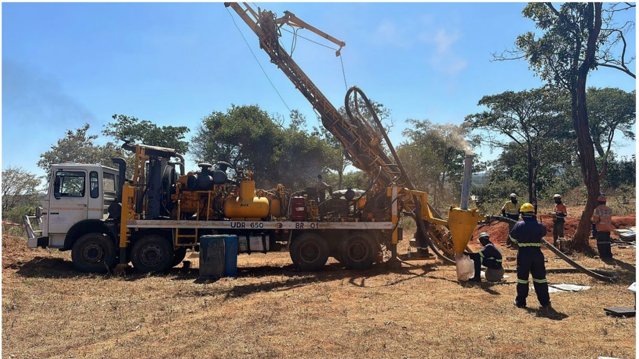
Figure 5: RC Drilling at Mpanda Project
