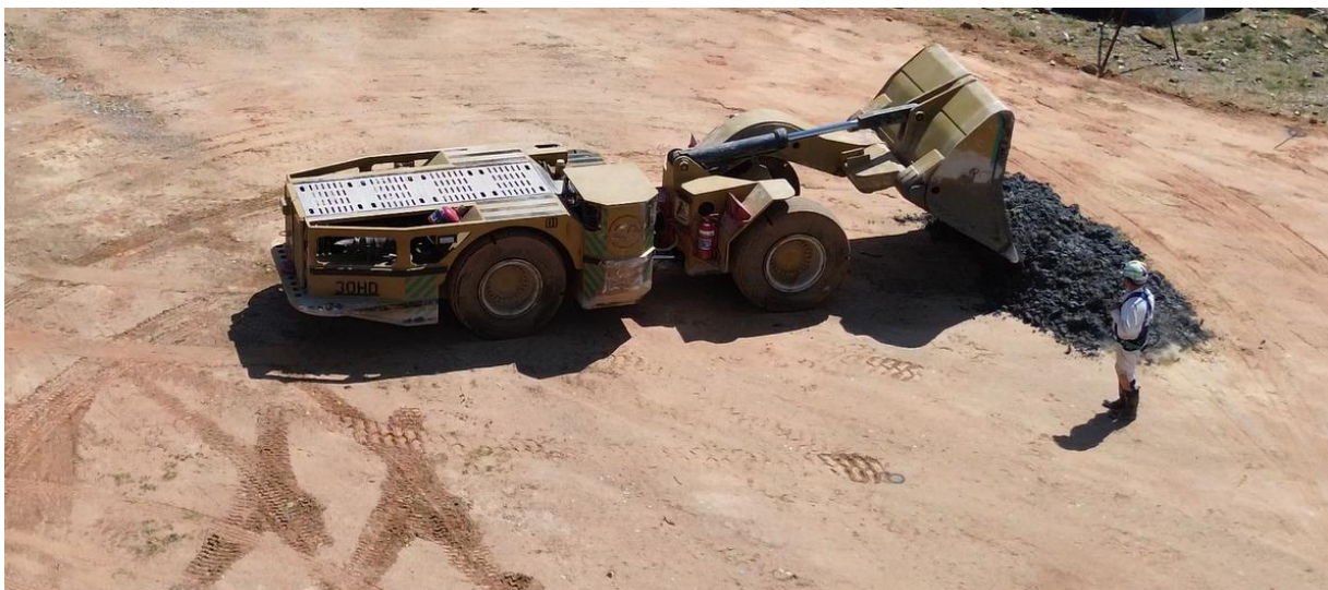
IMAGE 4: LHD DROPS FIRST ORE AS PRODUCTION ACTIVITY BEGINS TO RAMP UP ON SITE
