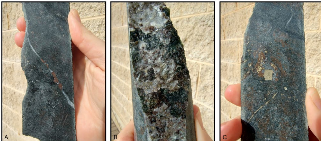
Figure 4. Photos of drill core from drillhole BUDD100, from left to right (A) disseminated chalcopyrite and bornite with sphalerite occurring along calcite veins (450.9m). (B) disseminated chalcopyrite and sphalerite (451.1m) and (C) disseminated chalcopyrite, pyrite, and sphalerite with pyrite and chalcopyrite veining (451.2m).
