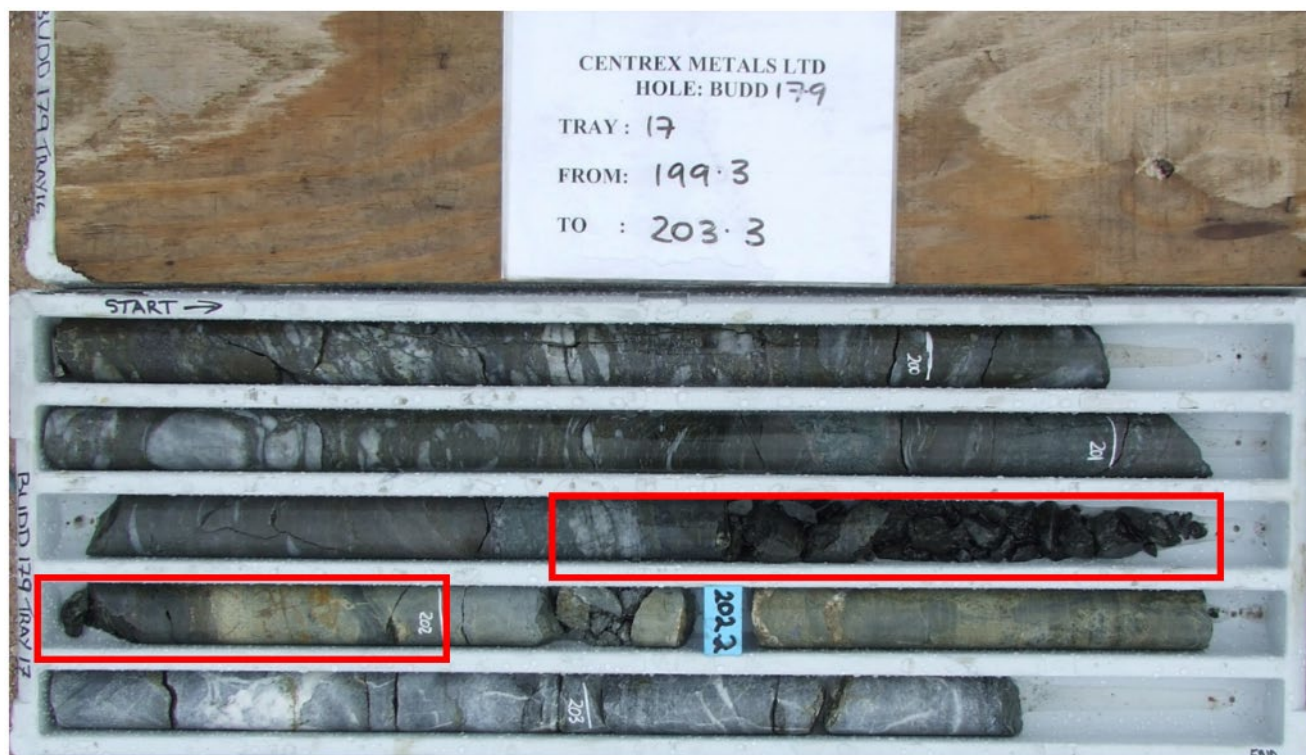
Figure 7. BUDD179 201.3-202m intercept where Pb-Zn mineralisation occurs within the sheared-out footwall of a larger breccia zone. The breccia zone contains massive pyroxenes and dolomitic marble.
