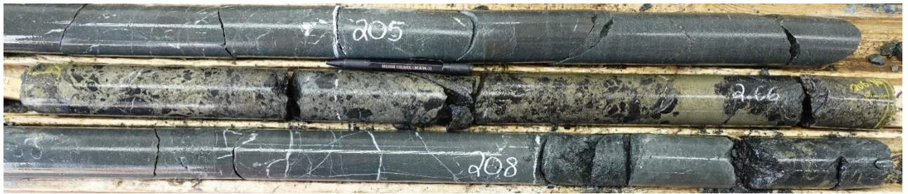
Figure 3: Brecciated Semi-massive VMS intercept 206.24-206.95m
