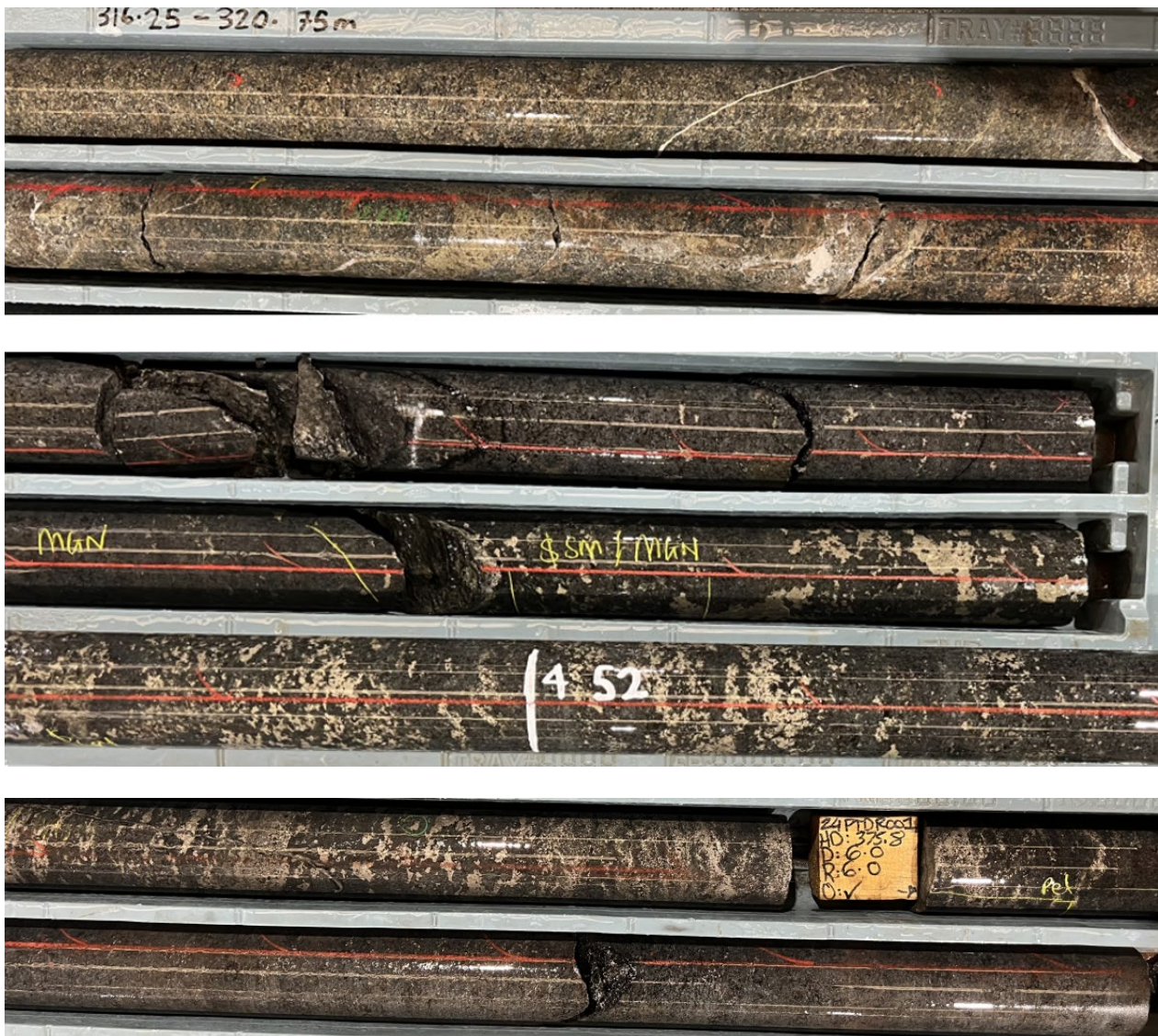
Figure 7: PP-GRAV02 diamond core drill hole 24PTDR001 potassic altered (biotite-amphibole-chlorite \pm minor K-spar, albite and calcite) mafic intrusive (dolerite) hosting variable zones of disseminated, semi-massive, brecciated pyrrhotite-pyrite-chalcopyrite copper mineralisation. NB: Scale = NQ diamond core diameter 48mm.
