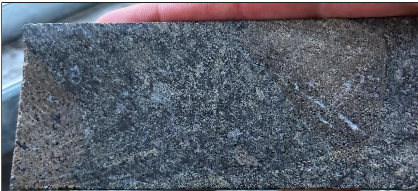
Figure 7. Core photograph from 412.2m to 414.2m in ZRSD25201 showing strong sphalerite with pyrite – 10.7g/t Au and 3.3% Zn.
