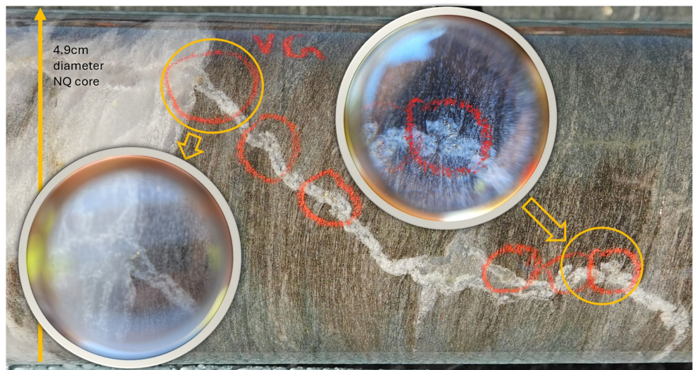
Figure 1. Bronzewing South, Eastern Boundary Target diamond drill-hole BWSRCD081 with visual gold logged at 416.8m down-hole from a 7cm wide zone within a 0.5cm wide quartz vein. Refer to Table 2 for observations.
