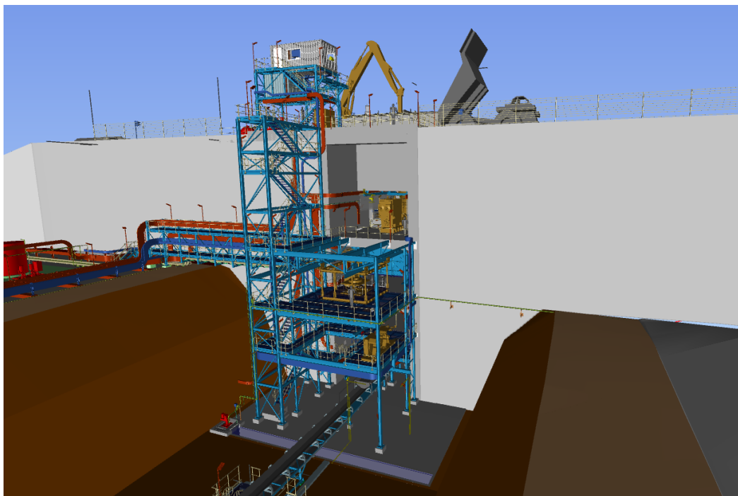
Figure 5: 3D model of primary crushing building and retaining wall
