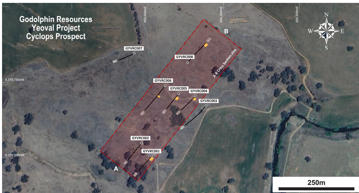
Figure 2: Location of drillholes at the Cyclops prospect
