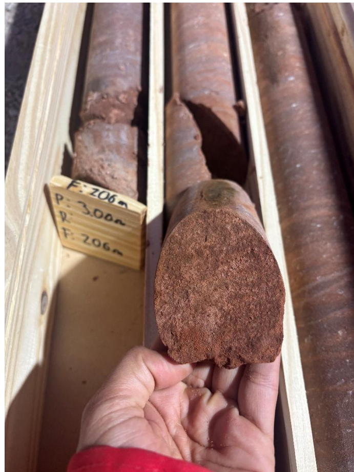
Figure 1. Jam25-05 core lithology at 206m showing clay units interspersed with sandy units and consolidated clay siltstone with specs of gypsum and anhydrite.
