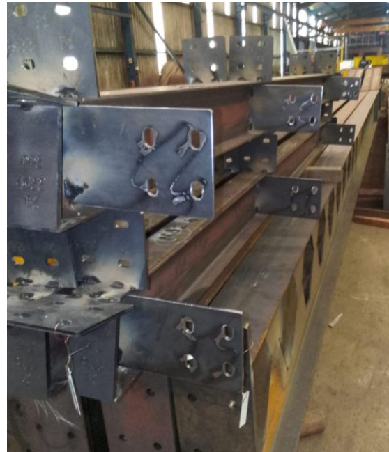
Figures 3 & 4: Steel plate (LHS) and structural steel (RHS) fabricated and ready for shipping to Kobada
