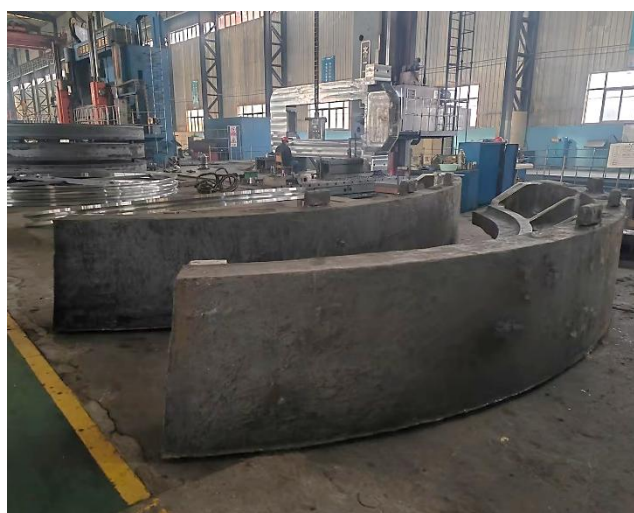
Figures 1 & 2: Components of the Kobada ball mill cast in the NCP factory - shell (LHS) and girth gear (RHS)
