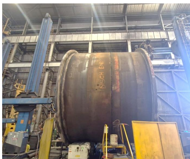
Figures 1 & 2: Components of the Kobada ball mill cast in the NCP factory - shell (LHS) and girth gear (RHS)
