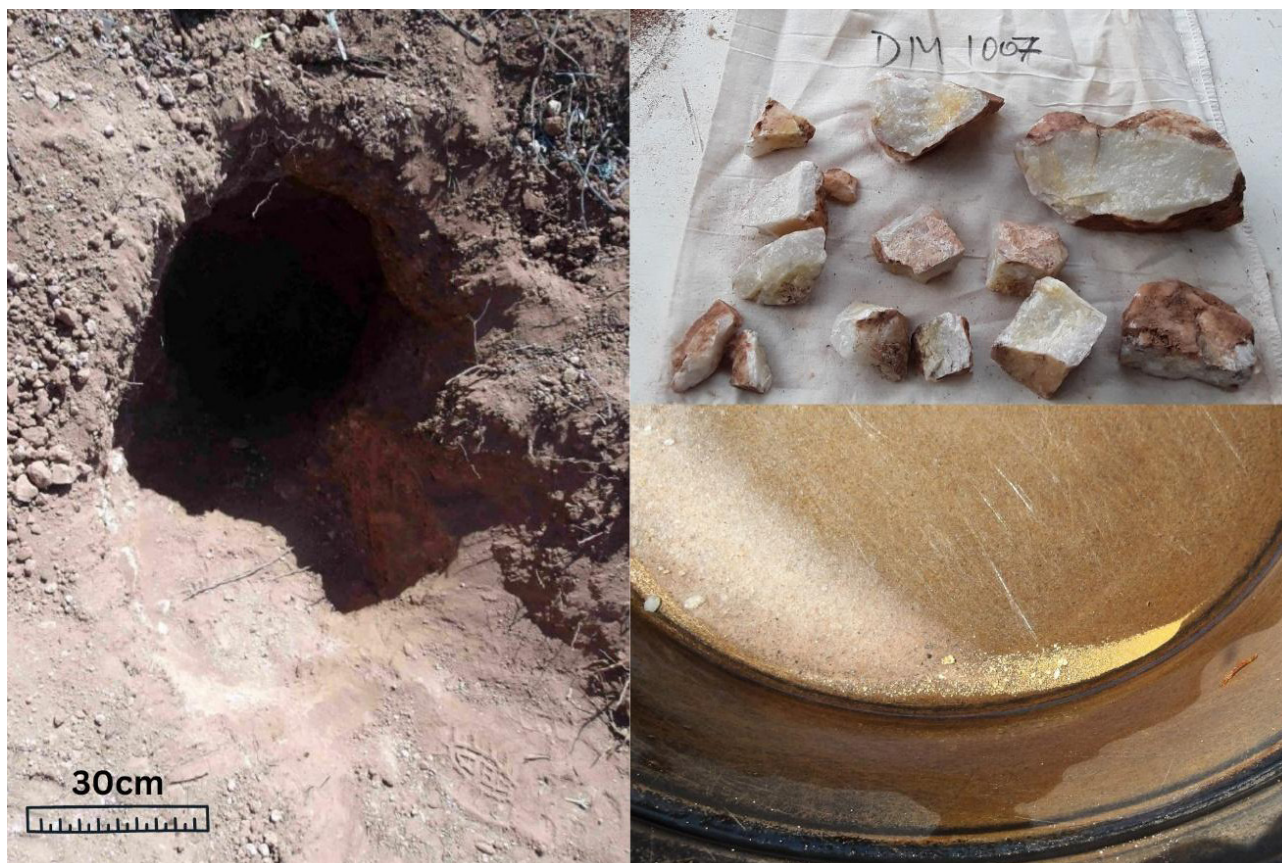
Figure 3. Sample DM1007 @ 2,040g/t Au. Hole from where DYM1007 was taken (left), quartz sample sent to lab (top right) and gold panned from dollied sample in the field
