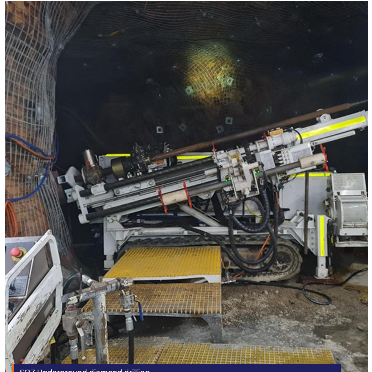
SOZ Underground diamond drilling
