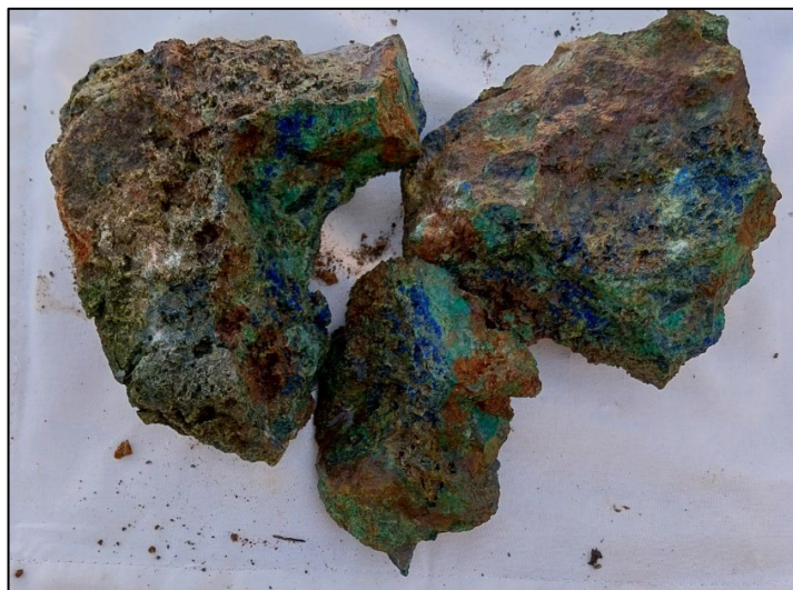
Figure 12. Sample PER056 collected near shallow workings at the central-southern portion of the Black Ridge trend during reconnaissance mapping. The sample contains secondary copper carbonates (blue and green) in an altered andesite host, with assays for the sample returning 7.5% Cu & 23g/t Ag (ASX MAG 26 September 2024).
