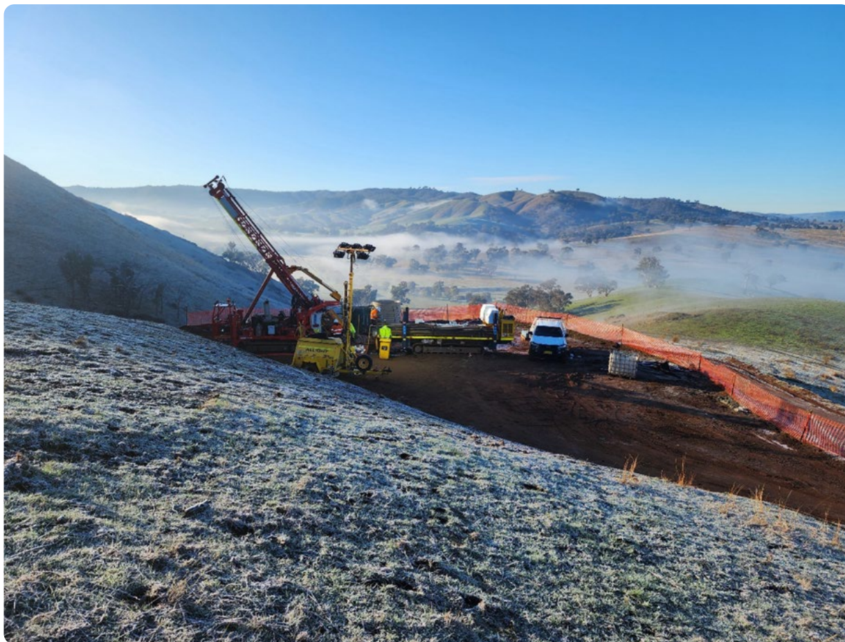
Figure 9 – Diamond drilling at Greater Hobbs Pipe in June 2025
