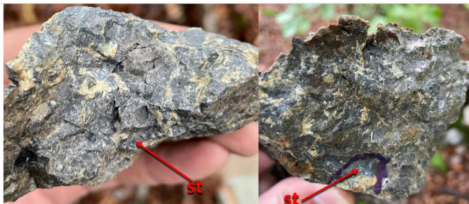
Figure 3. (above) Outcropping zone of stibnite mineralisation over 5 m wide at Kreva Prospect at east end of 3.3 km soil anomaly with Sb assay results indicated. (below) Close up of stibnite mineralisation 4 .
