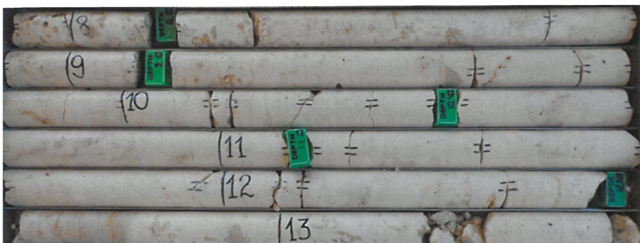
Fig 1 - Soalara Limestone Core - High purity @ 97% Calcium Carbonate
