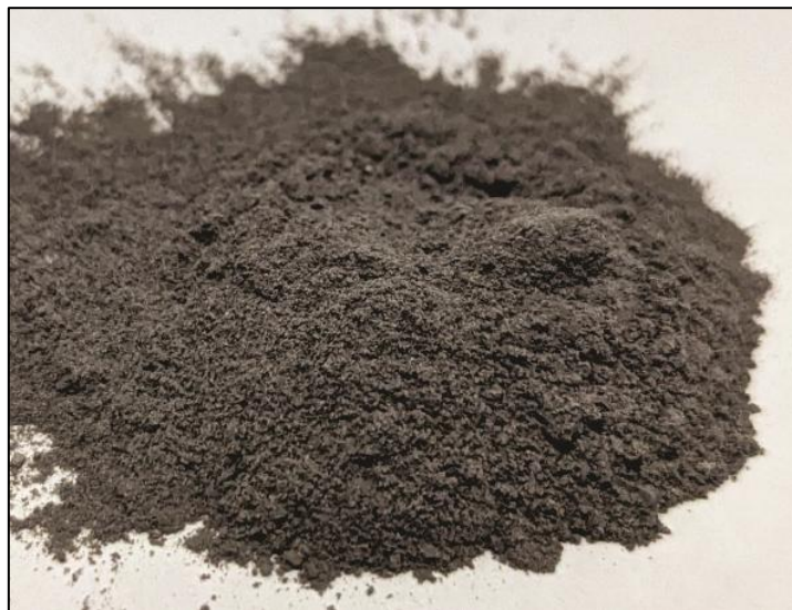
Figure 4: Antimony sulphide (37% Sb) precipitated from leach liquor 6
