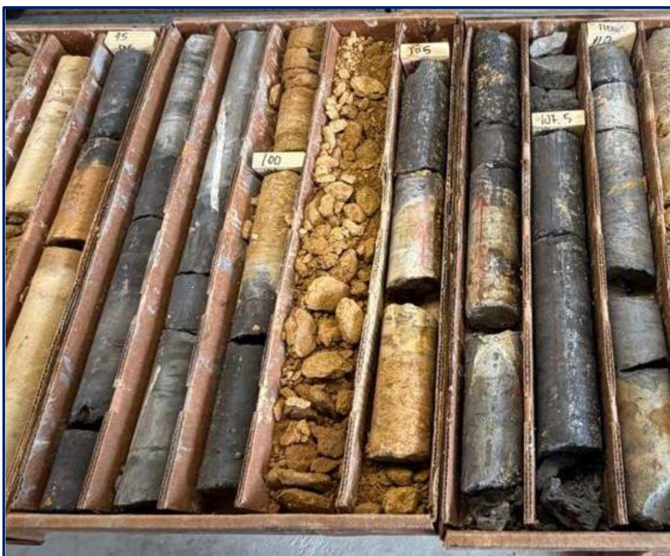
Figure 1 – Hole ACP26DD001 showing the main mineralised horizon between 95 and 110 feet downhole, comprising massive to semi-massive stibnite (estimated ~12% \text{Sb}_2\text{S}_3 ), underlain by a less mineralised conglomerate.
