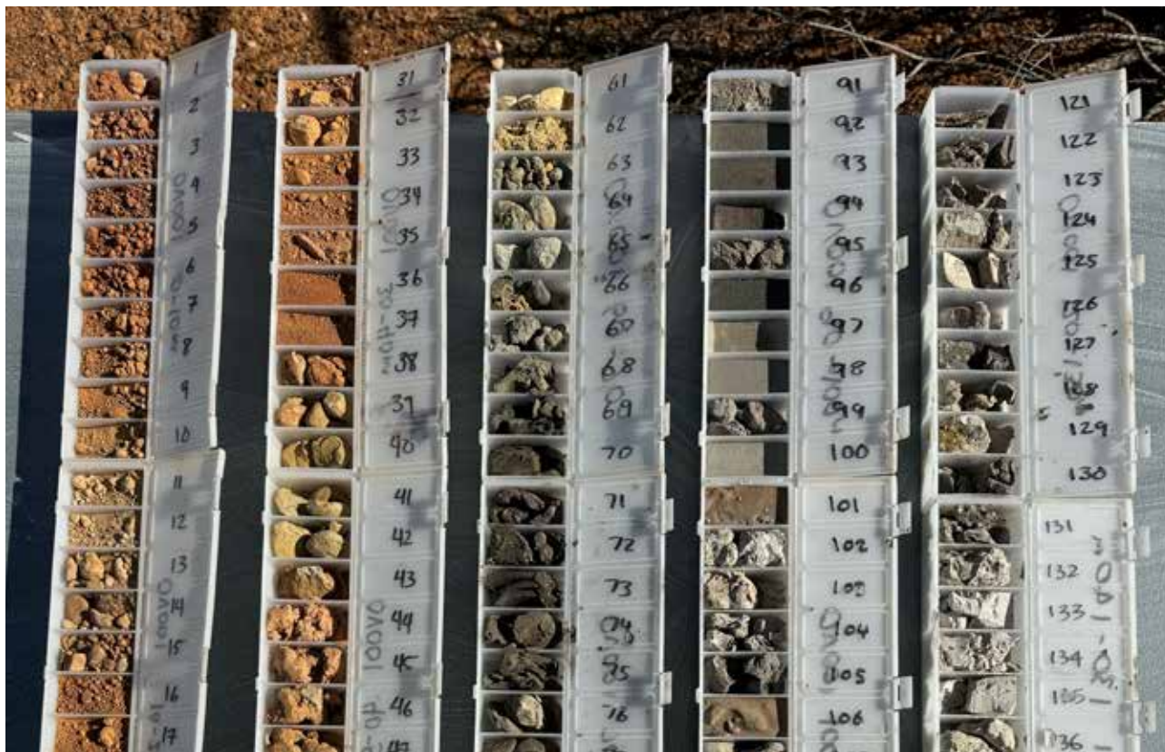
Overland drilling - 1m interval chip trays showing redox boundaries and ISR amenable sediments (OV001)
