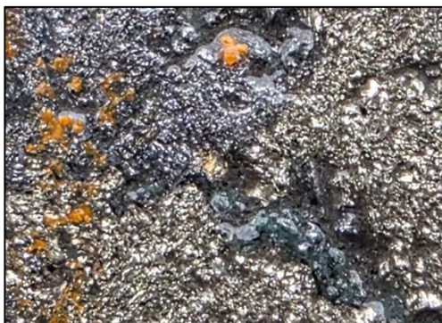
Image: Visible gold (1mm approx.) with pyrite, tetrahedrite and chlorite in drill hole SB-25-03.
