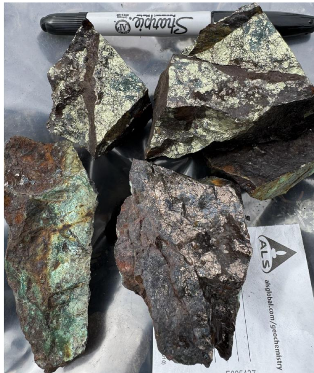
Figure 5: Photograph of sample F005437 with massive bornite-chalcopyrite which returned 42.60% Cu, 2.28g/t Au, 159g/t Ag, 0.364% Co from the Glacier IOCG trend.
